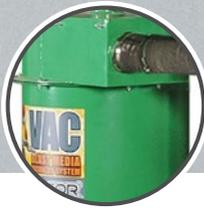
The blasting media is sucked in by the vacuum suction system via a stand-alone dust pre-separator SC-500 and the blasting media suitable for reuse is separated from the unusable medium.
